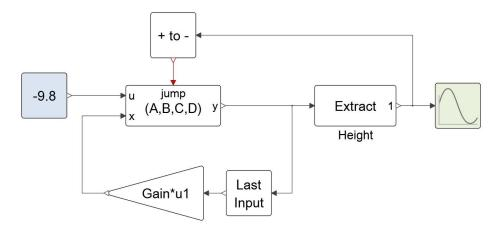
The output of the block JumpStateSpace is a vector of size two consisting of  $[x,v]^t$ . Whenever the condition (x < 0) is satisfied, an event is generated by the Zero-crossing (+ to - ) block. This event makes the Jump block do a reinitialization, *i. e.*, v := -0.9v and x := x. The Clock block generates periodic events (activation signals) to activate the Scope block which displays x and v.
